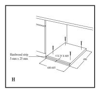
With the appliance installed adjust all four feet ensuring the machine is stable, and a clearance of approximately 5 mm is left between the top of the machine and the underside of the worktop.
